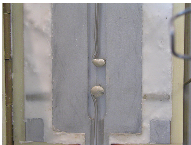
Fig. 1. Experimental set-up used to investigate the conductivity as a function of temperature. The fiber is connected to two electrodes with silver paste. The fiber is placed in a temperature controlled chamber, which is here opened. The strain is kept fixed during the measurements.
